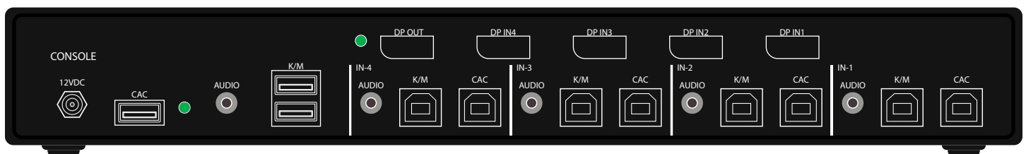
Figure 4-2: SA-DPN-4S-P Rear panel
